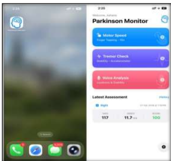
Figure 1: Parkinson Monitor application interface. Left: home screen deployment. Right: main dashboard displaying the Motor Speed, Tremor Check, and Voice Analysis modules alongside the most recent assessment summary.
